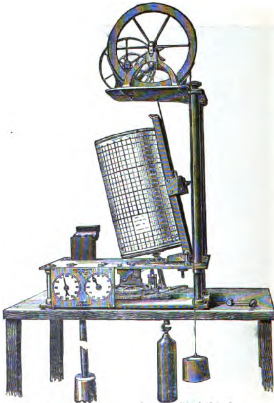
FIG. 117.—Tide-gauge for recording local tides, a pencil moved up and down by a float writes on a drum driven by clockwork.
